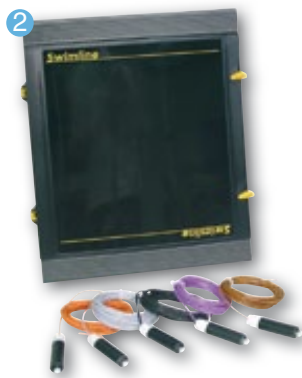
RED-2: Balance tank regulation control panel comprising 5 stainless steel sensors (ground, pump shut down, solenoid valve open and close, overflow safety) and a 20/27 brass solenoid valve. Protected by a fuse.
