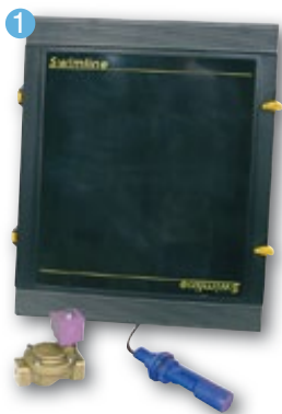
RED-1: Pool water level regulation control panel, comprising an adjustable level sensor, a timer and a brass 20/ 27 solenoid valve. Protected by a fuse.
